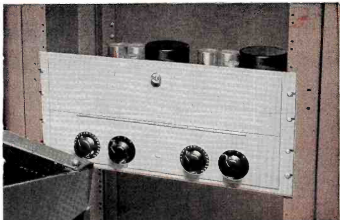
The RCA Type BR-2A Shelf fits any standard rack; takes 8 3/4 inches of panel space. If desired, however, RCA Type 36-B panels and shelves now in use can be easily adapted for plug-in amplifier service.
